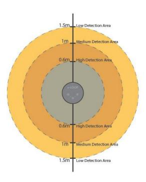
Varying magnetic field detection zones. The grey area depicts a 0.6m high sensitivity detection area surrounding the e-loop, suitable for the majority of vehicles. The dark colour area depicts a 1m medium sensitivity detection area surrounding the e-loop, suitable for most vehicles. The light colour area depicts a 1.5m low sensitivity detection area surrounding the e-loop, which is only suitable for some vehicles.
